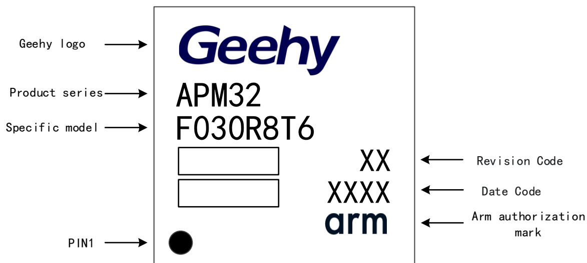
Figure 21 LQFP64 coding specification
